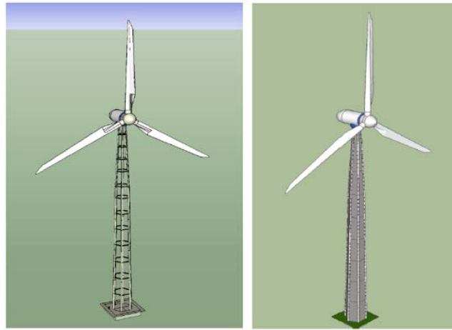
Figure 1.30. Lattice tower with horizontal bracing (left); horizontal tower with panel bracing (right) (Lewin & Sritharan, 2010)
