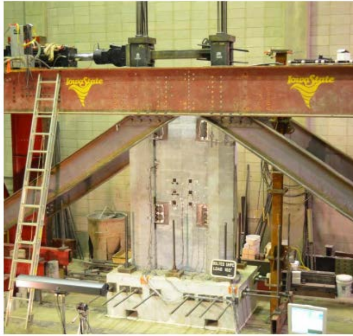
Figure 2.10. Test unit setup, bolted connection test (Schmitz, 2013)
