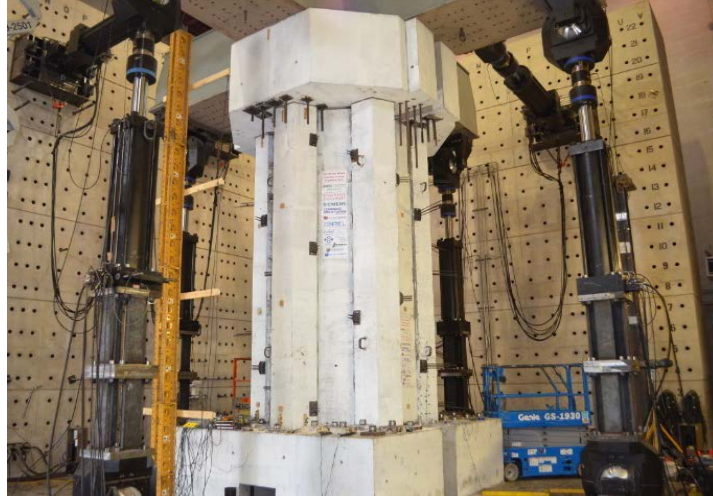
Figure 5.4. Hexcrete tower test unit
