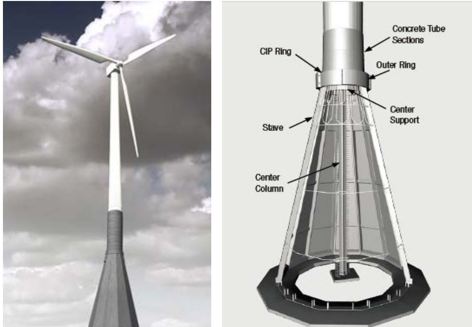
Figure 1.15. Tyndall Atlas CTB tower concept (left) and tower details (right) (Zavitz & Kirkley, 2016)
