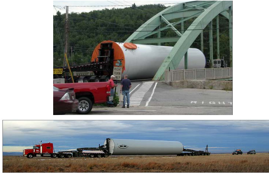
Figure 1.7. 80-m wind tower barely fits under bridge (top) (Sun Journal, n.d.); 80-m standard wind tower transportation (bottom) (National Renewable Energy Labs (NREL), 2009)
