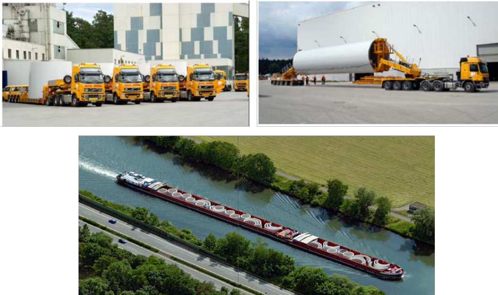
Figure 1.23. Transportation of wind tower components: concrete sections (upper left); steel section (upper right); concrete sections via ship (lower)
